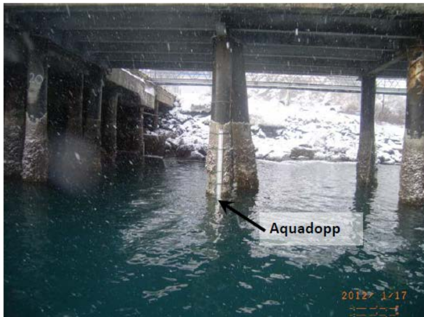
Figure A2. Aquadopp Instrument attached to dock pile for wave and current field measurements
