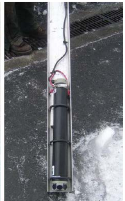
Figure A2. Aquadopp Instrument attached to dock pile for wave and current field measurements
